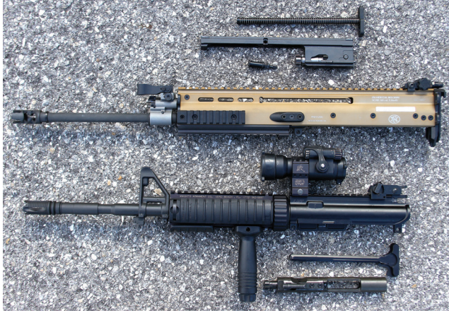
Figure 4.66 A contrast between the upper receivers of the FN SCAR 16S (top) and an AR-15 (bottom). The bolt carrier groups have been removed to contrast the differences between the two. The SCAR is operated by gas piston; the AR uses the traditional gas impingement. Installed on the AR upper receiver is a Knight's Armament RAS free-floating rail system, an aftermarket flash hider, a MaTech rear sight, a Knight's Armament vertical fore grip, and an Aimpoint Comp M4 using a Knight's Armament mount. (Image from author's collection.)
